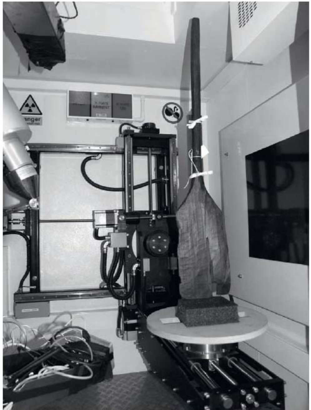
Fig. 1. Photograph of a spade from Oseberg ready to be scanned. The spade is mounted on an upright by means of cotton tapes.
