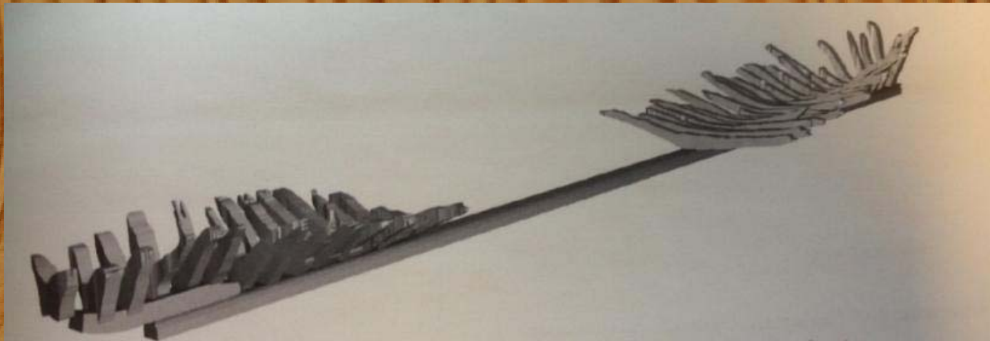
Tri-dimensional model of ship`s frames, in Castro, F., Yamafune, K., Eginton, C. & Derryberry, T. (2011). “The Cais do Sodré Shipwreck Lisbon, Portugal” . Centre for Maritime Archaeology and Conservation, Department of Anthropology, Texas A & M University, College Station. The international Journal of Nautical Archaeology ,40:2:, p. 343
