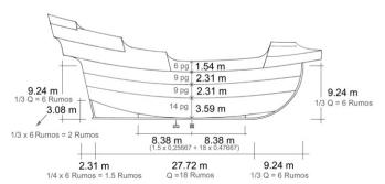
**Fig. 4.** A profile of the Pepper Wreck with some of the measurements indicated in Oliveira's treatise and the presumed positions of the ship's decks. The measurements indicated do not include the thickness of the pavements, which was slightly over 1 *palmo de goa* per deck (Filipe Castro).
