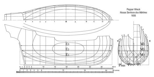
Fig. 6. Basic measurements of the reconstructed Pepper Wreck (Filipe Castro).
