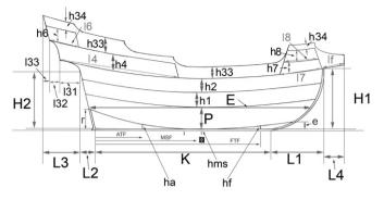
**Fig. 5.** Defining dimensions of an Iberian ship in the period under analysis, see Table 1 for explanations of the measurements indicated (Filipe Castro).
