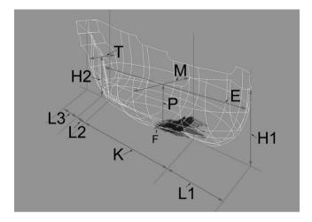
**Fig. 1.** Basic diagnostic dimensions of a ship: K - Keel length, L1 - Spring of the stem post, L2 - Rake of the stempost, L3 - Span of the counters and stern castle bulworks, H1 - Height of the stem post, H2 - Height of the sternpost, T - Width of the transom, M - Maximum beam (in Spanish*Manga*), F - Flat amidships (in Spanish*Plan*), P - Depth of hold (in Spanish*Puntal*), and E - Length on the upper deck (in Spanish*Eslora*) (Kevin Gnadinger and Filipe Castro).
